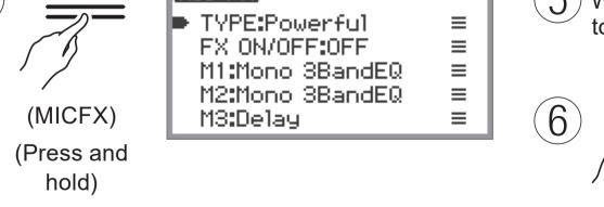
When "FX ON/OFF:OFF" is displayed, switch to ON.
