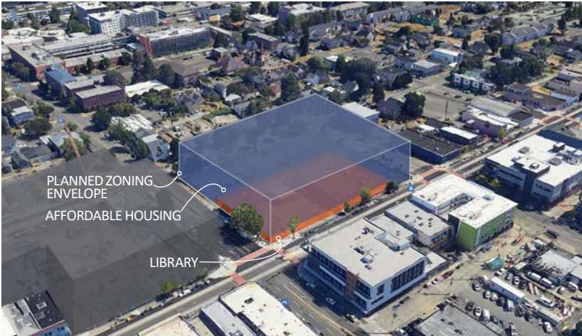
Figure 128. Option 2: Massing diagram of building.
